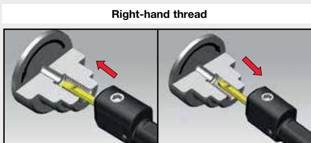
Insert: Right-hand design Direction of rotation: Clockwise M3 turning from outside in
