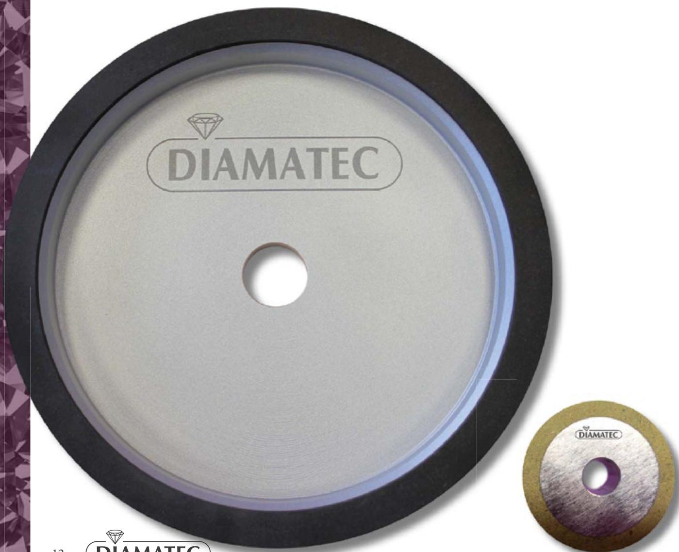
The advantage of vitrified Diamond or CBN wheels is the manufacturing process which permit to control the porosity of abrasive layer. This porosity permits to have empty spaces between grits to limit the surface in contact with the material, to reduce the cutting force and to maximize the circulation of the liquid.
